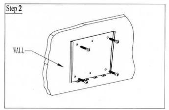
Step 2: Screw four lag bolts into the plastic concrete anchors through the wall dead plate to make the dead plate and vertical wall into a whole.
